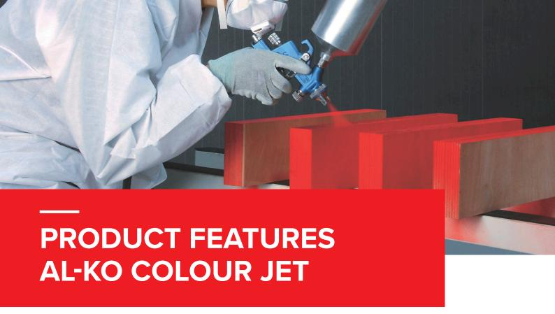
The devices of the COLOUR JET series are optimally designed for the extraction of paint mists and solvents at wet painting workstations.
